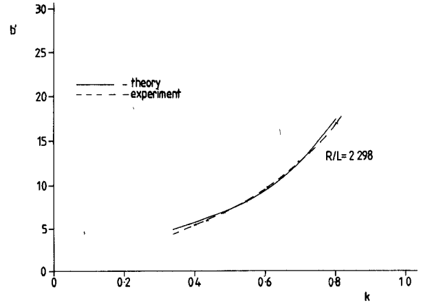
Fig. 9. Normalized susceptance slope parameter of single quarter-wave-long resonator [9].
